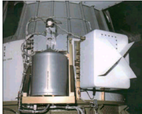
Figure 11. SEDS-1 on Delta II 2nd Stage
